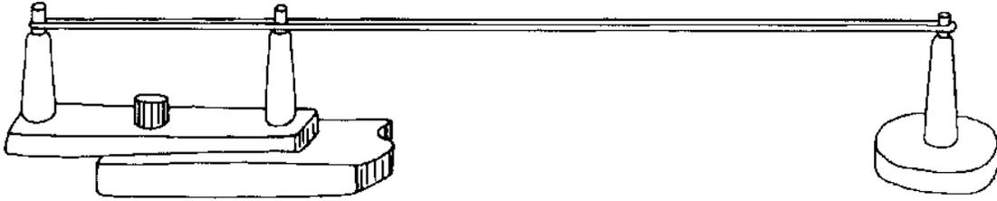
A simple portable wooden string jig can be clamped onto a table or work bench.
